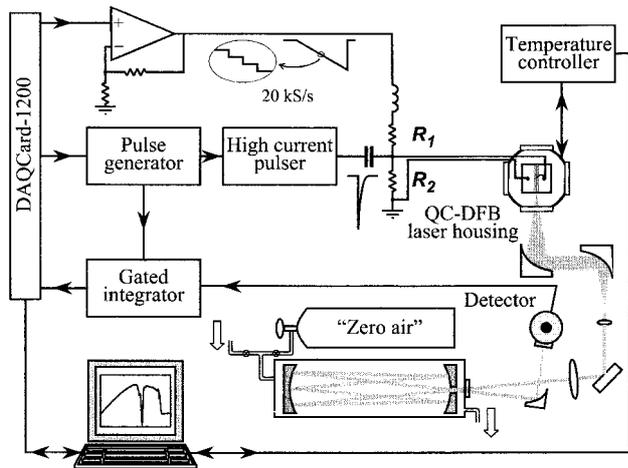
Fig. 1. Experimental arrangement for absorption spectroscopy with a pulsed QC-DFB laser. The laser is mounted on a thermoelectric cooler in an evacuated housing.
