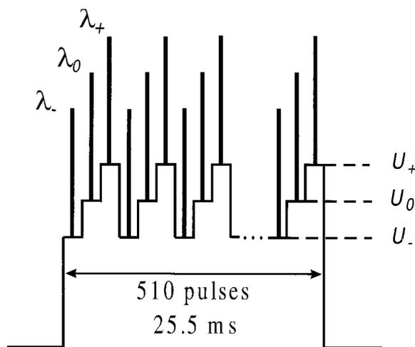
Fig. 6. Schematic of computer-controlled wavelength cycling for a pulsed QC-DFB laser. The steps show a subthreshold current (controlled by the computer-synthesized voltage U<sub>i</sub>) added to the short laser excitation pulses represented as spikes. The laser wavelength cycles through three temperature-dependent values λ<sub>i</sub>.
