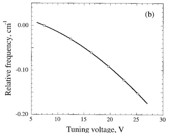
Fig. 2. Laser frequency: tuning (a) with temperature and (b) with a computer-controlled voltage applied to the resistor  $R_1$  (shown in Fig. 1). The circles show the positions of the etalon fringes used for calibration.
